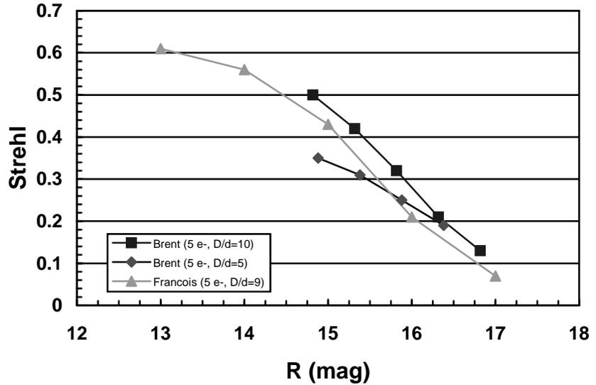
Figure 1 - Results of the Shack-Hartmann model comparisons are plotted. For comparable numbers of subpupils, the predicted performances of Brent's and Francois' models are quite close.
