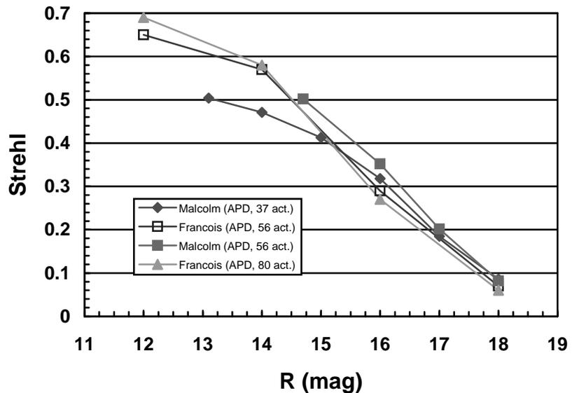
Figure 2 - Comparisons of all the curvature models are presented. All of the models yield comparable performance for stars fainter than R ~ 17 mag.
