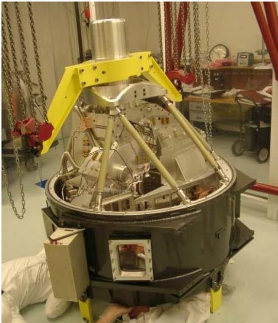
Figure 15 - The GNIRS cold structure held vertically by a crane in the NOAO clean room is shown as it is being lowered into the bulkhead assembly.
