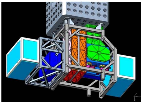
Figure 17 – NICI is shown mounted on the uplooking ISS port. The instrument is split into a warm AO front end that feeds a dual imaging camera. Three thermal enclosures are used to house all of the mechanism control electronics, bimorph drive electronics, a pair of array controllers, and all of the APD power supplies.
