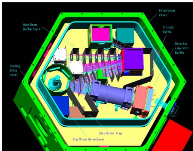
Figure 13 – The NIFS science channel is shown. The IFU feeds a turret (left side of assembly) containing a selection of gratings that are tuned to provide J, H, or K-band sampling at  $R \sim 5000$  in a single integration using a HAWAII-2 HgCdTe detector. This detector is housed in the structure to the lower right, within the cold light shield that contains all of the optics and mechanisms.
