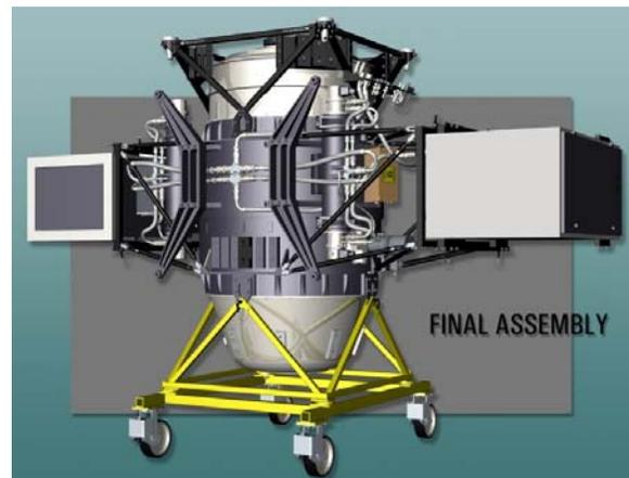
Figure 16 – A CAD rendering of the completed GNIRS in an up-looking mode is shown. The central bulkhead seen in Figure 15 ties together the other vacuum jacket sections, electronics enclosures, and ISS interface plates.
