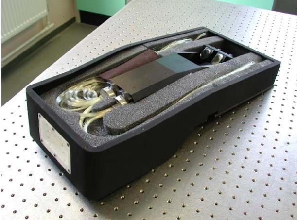
Figure 4 – The GMOS IFU is shown with its top protective case removed. A pair of pick-off mirrors are seen on one end, with the 1500 fibers arching within the assembly, suspended by foam lining to provide a protective low stress environment.
