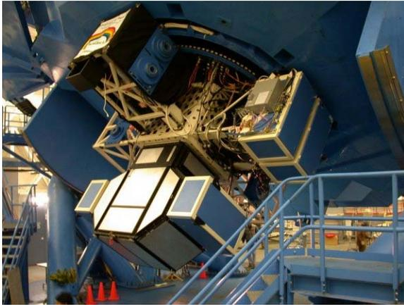
Figure 3 – GMOS is shown on the up-looking port at Gemini-N. Like NIRI, prominent in the physical layout of the instrument are the 2 outrigger thermally insulated electronic cabinets that serve to remove heat from the instrument, through facility glycol lines, which is routed to the outside by a large chiller. The instrument's shiny outer panels serve to buffer the inner GMOS opto-mechanical structure from temperature variations outside.
