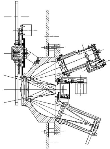
Figure 7 – A cross section of the novel GCAL integrating hemisphere is shown, which injects a beam of light generated by one of several sources into the main projection mirrors.
