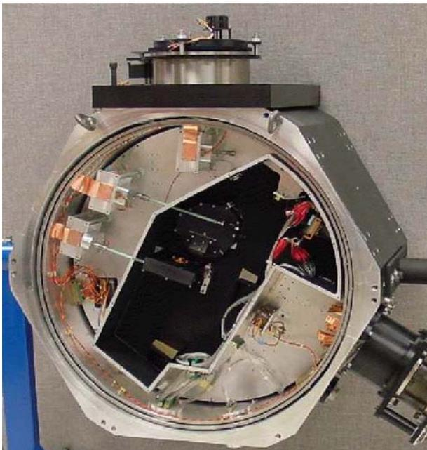
Figure 9 – A view of T-ReCS from the “bottom” is shown. Cryomotors are seen with fiberglass feed-throughs into the central light-tight baffle box, which contains various optical elements.
