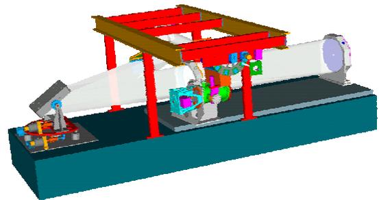
Figure 11 – A CAD rendering of the completed bench spectrograph is shown. This is Gemini’s only fiber fed instrument, which is capable of high stability spectroscopy at fairly high resolution across optical wavelengths.
