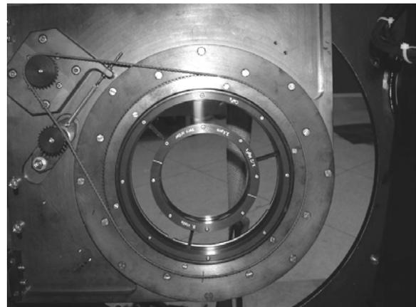
Figure 8 – A picture of one of the waveplates in GPOL, when deployed into the telescope beam, is shown. The waveplate is in the center circular cell and is immediately surrounded by an annulus of fused silica, which the OIWFS in an instrument uses to find guide stars.
