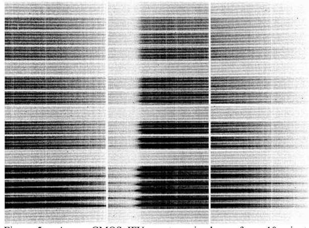
Figure 5 – A raw GMOS IFU spectrum is shown for a 10 minute integration on M32. The bright vertical lines which split the field in thirds are the CCD mosaic gaps. Sky lines from the 500 fiber outrigger are the relatively light (low signal) horizontal bars which divide the field into fifths.
