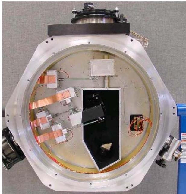
Figure 10 – Same as Figure 9 but the view from the “top” of the instrument is shown. At the top of the vacuum jacket is seen the novel window rotating mechanism which puts 1 of 5 windows into the beam.
