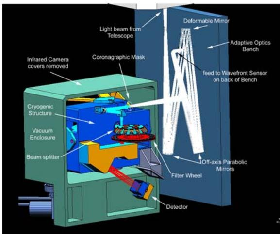
Figure 18 – The two principal components in the NICI optomechanical assembly are shown. The AO bench, which houses and 85 element curvature wavefront sensor, is shown only schematically here.
