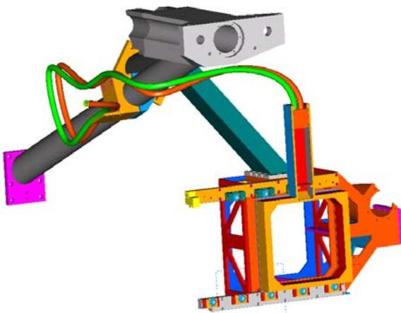
Figure 12 – The GMOS module that contains the fiber entrance feed for bHROS is shown. This module inserts within the GMOS mask exchange mechanism like an IFU, meaning GMOS can be configured to rapidly support straight through imaging, MOS spectroscopy, bHROS spectroscopy, or integral field spectroscopy, through remote control.
