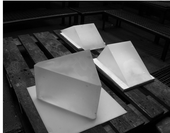
Figure 8 - Large rough-cut fused silica intended for use in HROS is shown.
