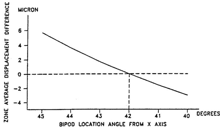
Figure 16. Zone displacement variation versus bipod location angle
