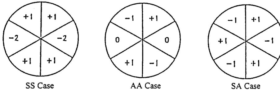
Figure 11. Patterns of force variation on mirror in the 6-zone hydraulic support system
