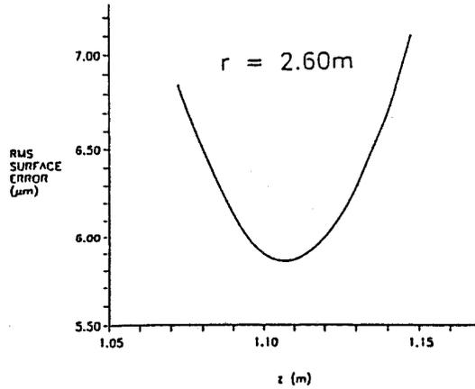
Figure 13. Cell deformation versus bipod location in Z at horizon pointing
