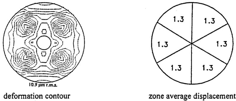
Figure 14. Cell top surface deformation at zenith pointing
