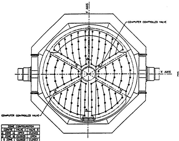
Figure 2. A schematic of the 3-zone / 6-zone hydraulic support system
