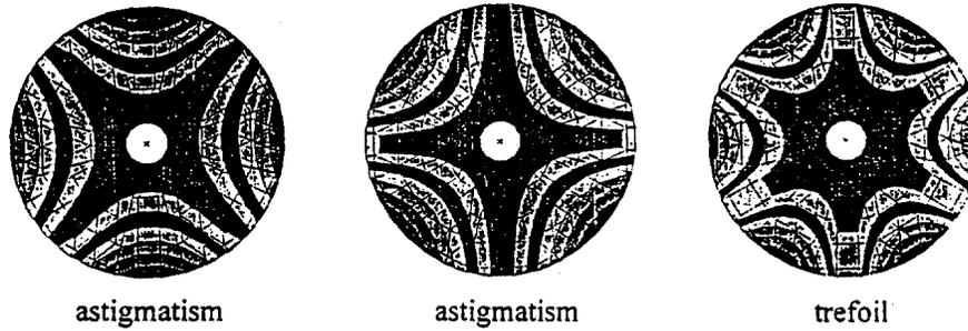
Figure 10. Three coupling modes in the 6-zone hydraulic support system
