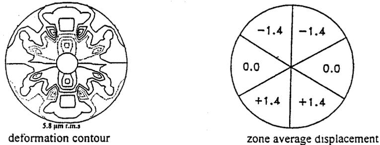
Figure 12. Cell top surface deformation at horizon pointing
