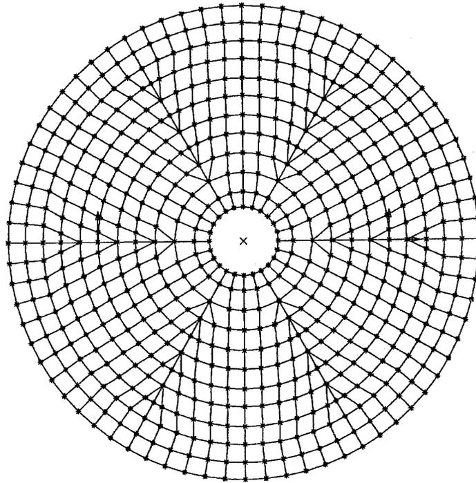
Figure 1. Finite element model of the primary mirror.
