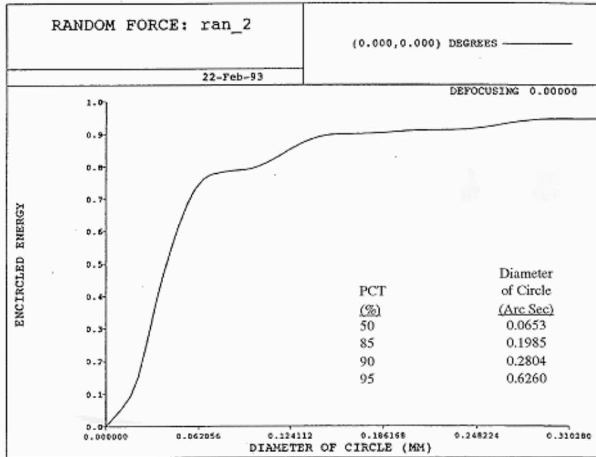
Figure 4. Typical encircled energy distribution.
