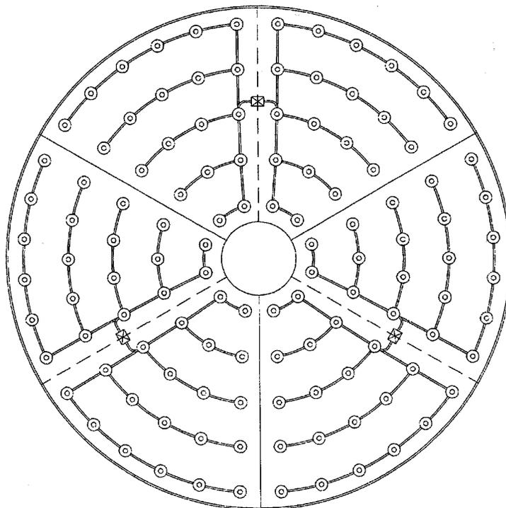
Figure 2. Six-zone hydraulic whiffle-tree defining support system
