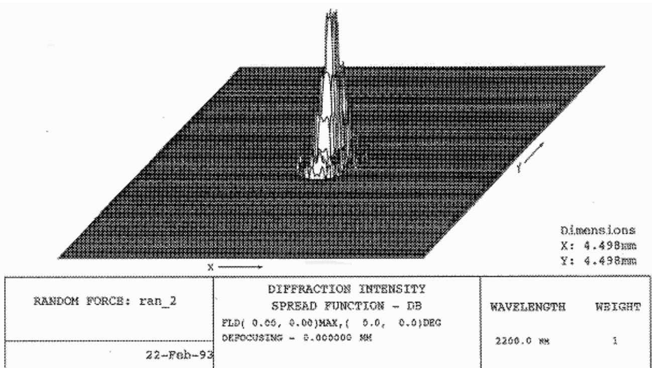
Figure 5. Typical plot of Point Spread Function.
