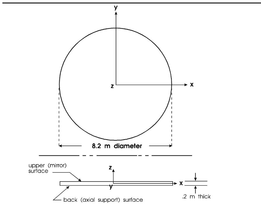
**Figure 1.** Simplified geometry for the meniscus mirror.
