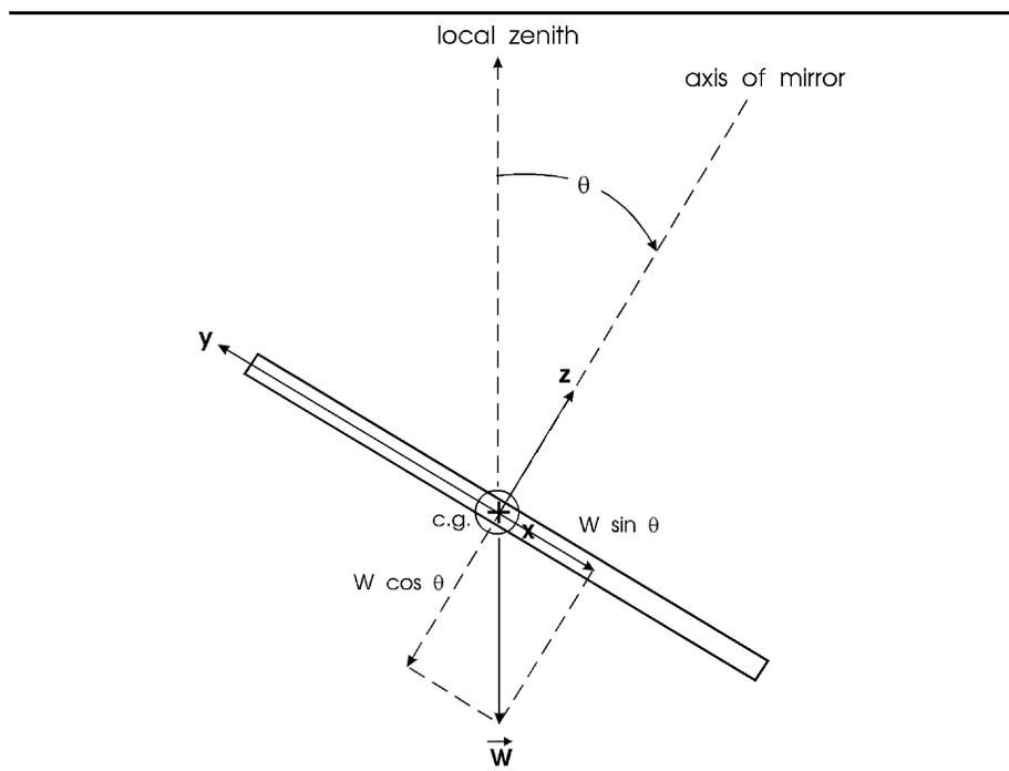
**Figure 2.** The mirror in relation to the gravity-weight vector,  $W$ .
