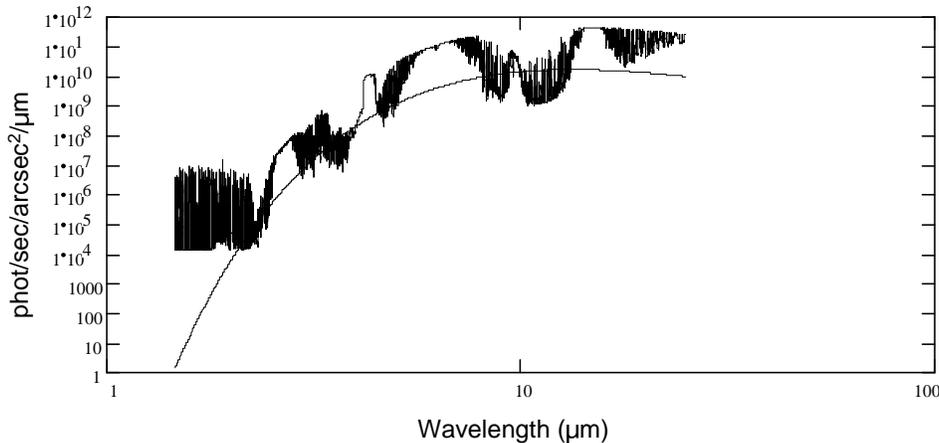
Figure 2.2 - Plots of F<sub>λ</sub> vs. λ for the atmosphere and telescope are plotted in units of photons/sec/arcsec<sup>2</sup> at the Gemini focal plane.
