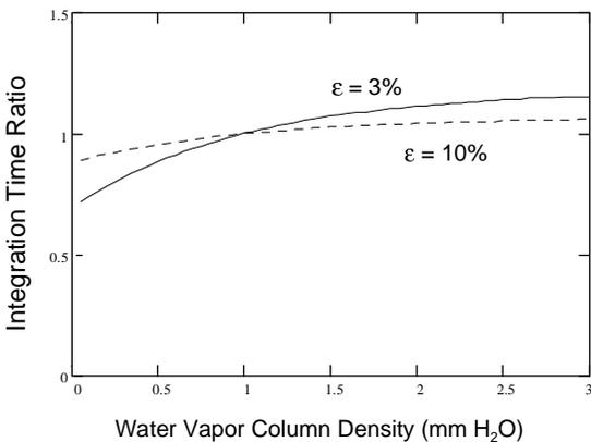
Figure 2.3 - Relative integration times for observations in the 3.8 and 11  $\mu\text{m}$  windows for telescope emissivities of 3 and 10% are shown. Integration time ratios are normalized to the value at 1 mm  $\text{H}_2\text{O}$ .
