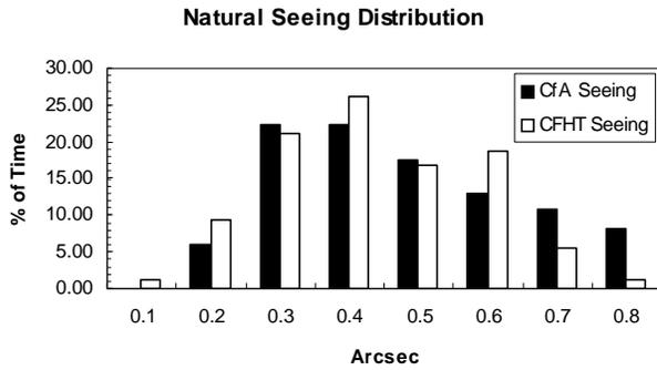
Figure 3.1 - A histogram distribution of seeing at the CfA and the CFHT is shown. Note that though the CfA monitor runs continuously, only night-time measurements are included in this histogram and the CfA data beyond 0.8" have been clipped to mimic the selection effect evident in the CFHT data (i.e., seeing measurements are not made during cloudy conditions).
