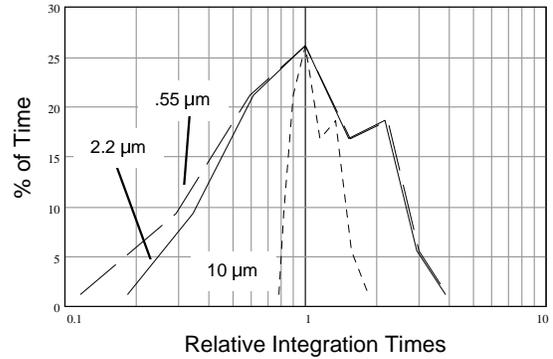
Figure 3.3 - Relative integration times at 3 wavelengths given Mauna Kea seeing distributions are plotted. Diffraction effects make 10  $\mu\text{m}$  imaging least susceptible to variations in seeing.
