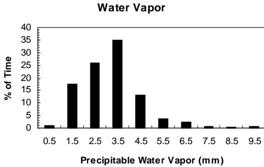
Figure 2.6 - A histogram of water vapor measurements made with the CSO  $\tau$  meter is shown for 100 nights. The conversion between 225 GHz opacity and precipitable water vapor was provided by Colin Masson (1992, Proceedings of IAU Colloquium No. 140, "Astronomy with Millimeter and Submillimeter Wave Interferometry").
