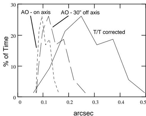
Figure 4.1 - A plot of the distribution of AO corrected image quality at 2.2  $\mu\text{m}$  is shown for stars on axis (short-dash) and 30" off axis (long dash). The solid line corresponds to tip/tilt corrected.
