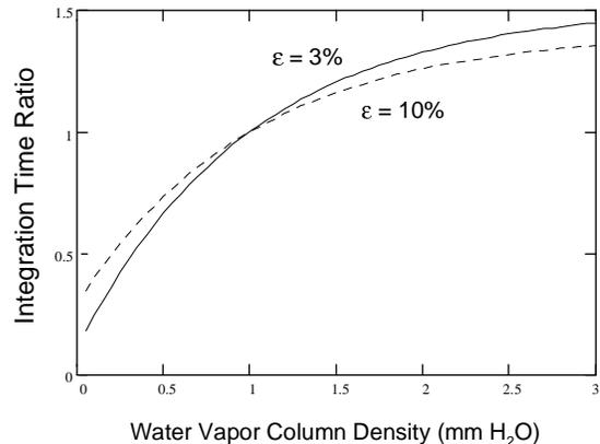
Figure 2.4 - Same as Figure 2.3 except the 20  $\mu\text{m}$  case is shown. Note how large the variations in integration times are to reach a desired S/N ratio when the telescope emissivity approaches Gemini's goal of 2%.
