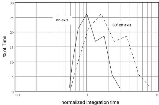
Figure 4.2 - The relative integration times at  $2.2 \mu\text{m}$  for on and off axis AO corrected stars is shown.
