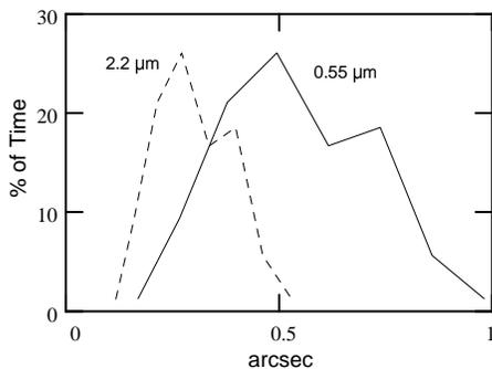
Figure 3.2 - Predicted delivered imaged quality distributions for Gemini at 2.2 and 0.55  $\mu\text{m}$  are shown. Gemini will clearly be much more susceptible to optical than infrared variations.
